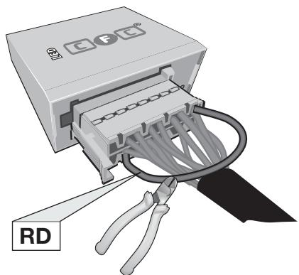
Pin 11 and Pin 2 disconnected
